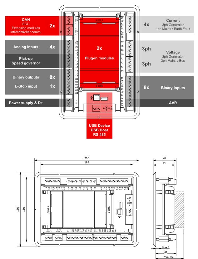
**Note:** The final depth of the controller depends on the selected extension module - it can vary between 41 and 56 mm. Mind also a size of connector and cables (e.g. in case of RS232 connector add about another 60 mm for standard RS232 connector and cable).
